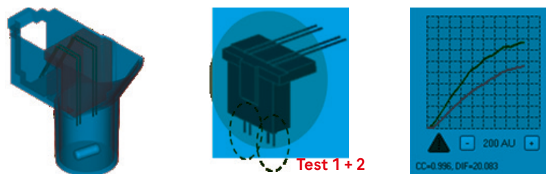
Figure 3. Two sensor test cell, for simultaneous determination of aggregation. The analyzer automatically compares signals and gives an error message if the difference is too high
